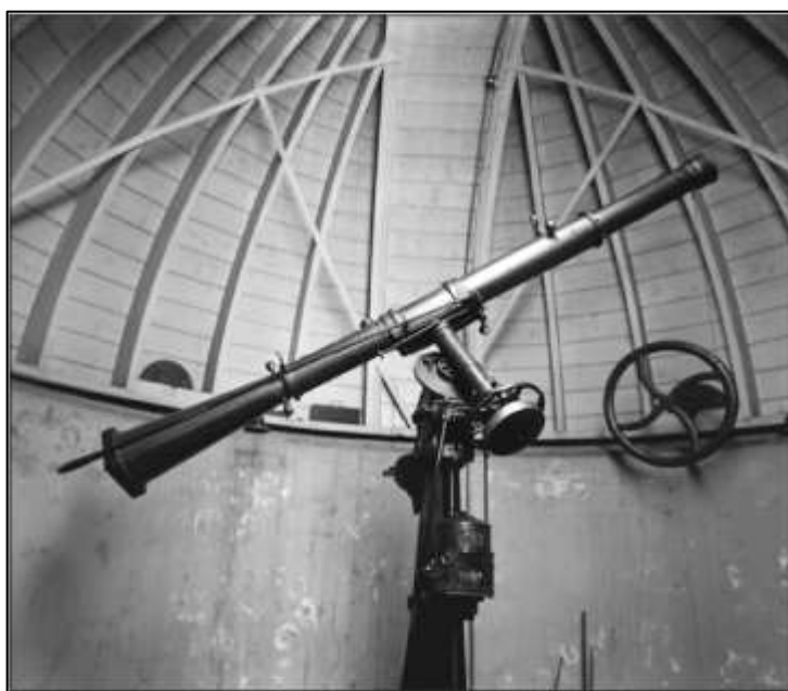
The 4 in Dallmeyer photoheliograph at Melbourne Observatory Courtesy Dr Barry Clark
